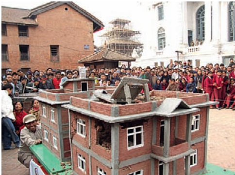
Fig. 2. Shake Table Demonstration for Masons, Policy Makers, Law Makers, Engineers, Technicians, General Public, and School Students to Make Them Understand the Performance of Buildings with Small Improvement in Construction (photo taken by NSET).
